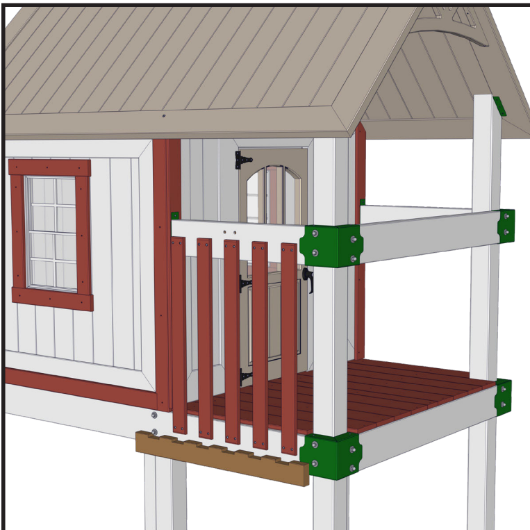
Step 35. Start installing the play slats using the included spacer. Fasten them using 1 3/4" washer head screws. The side with the swing frame gets five slats.
