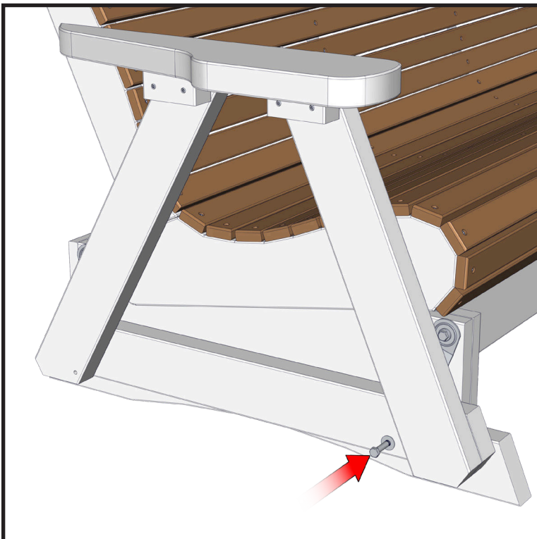
Step 19. Fasten the front bearing arm through the predrilled hole using a 2 1/2" hex head bolt with a nut and washer.
