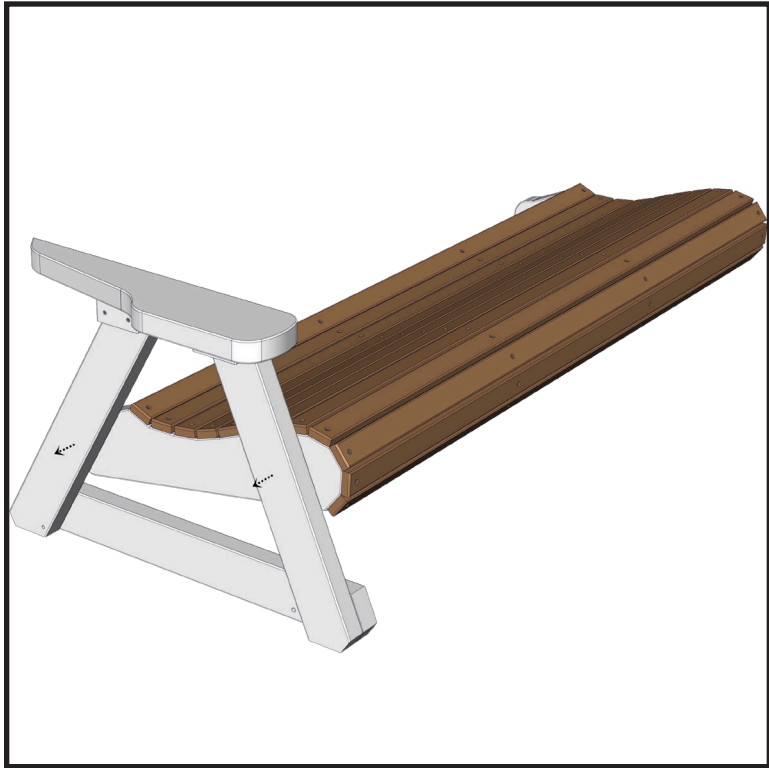
Step 10. Place the arm rest next to the seat assembly and align the holes.
