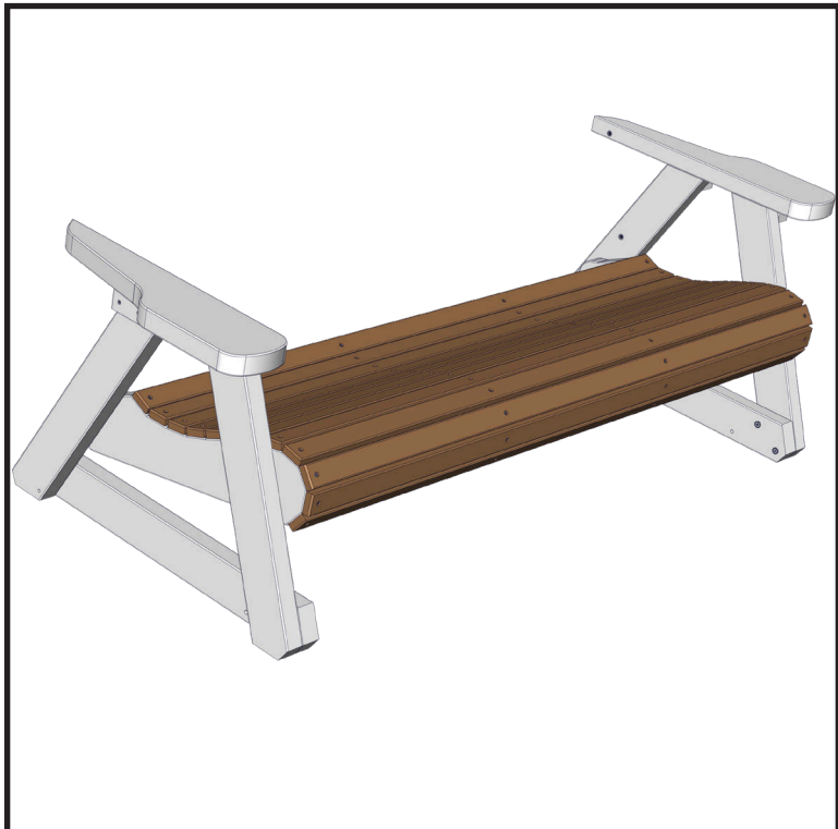
Step 12. Repeat the previous steps to install the other arm rest.
