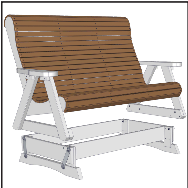
Step 18. Place the seat assembly over the base and align the bearing arms.
