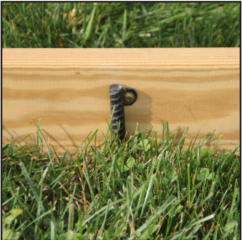
Playset Stakes Drive the stakes into the ground at each corner of the playset and fasten them with the included lags.
